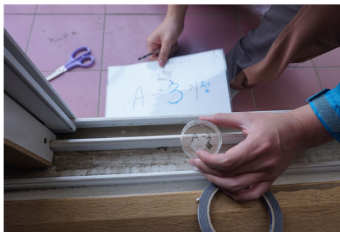
e) deposited dust collection and SEM/EDS analysis
