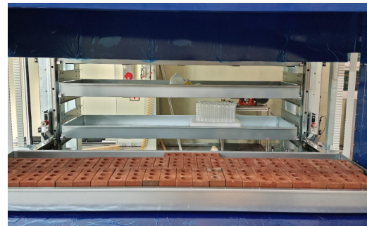
Fig. 8. Experiments to Improve Tray Deflections
