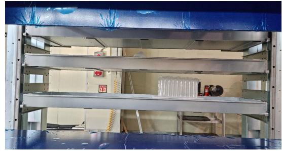
Fig. 7. The Two-Stage Palette for Simultaneous Receiving and Forwarding
