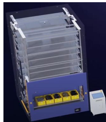
Fig. 4. Elevator Type Automatic Storage
