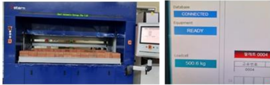
Fig. 17. Payload Test and Results Screen
