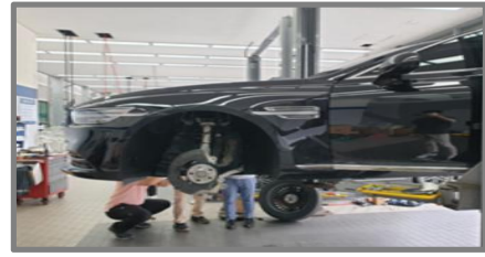
Fig. 12. Embedded system and 3-axis vibration sensor attachment process for actual vehicle driving test
