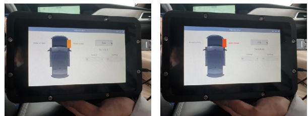
Fig. 13. Wheel bearing failure diagnosis module performance verification results
