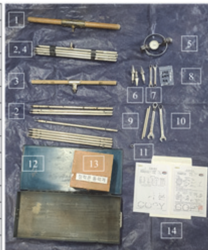
Fig. 1 Components of PSCPT equipment
