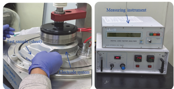
Fig. 9. Measuring tanδ of XLPE insulation.
