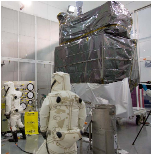
Fig. 1. Examples of Fueling Hydrazine Operation [14]
