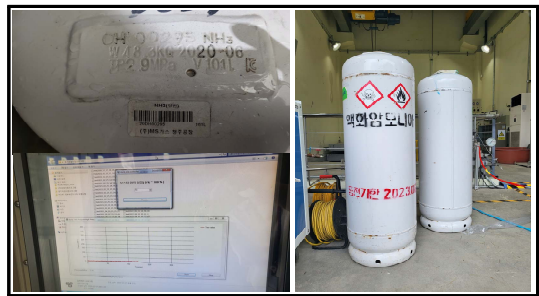
Fig. 2. Ammonia cylinder before hydraulic rupture test
