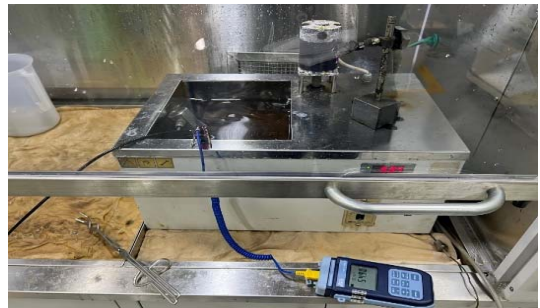
Fig. 5. Fusible metal type safety valve Activation test equipment
