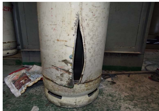
Fig. 1. Rupture accident cylinder
