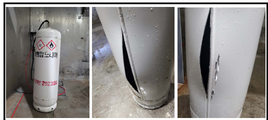
Fig. 3. Ruptured cylinder after hydraulic test
