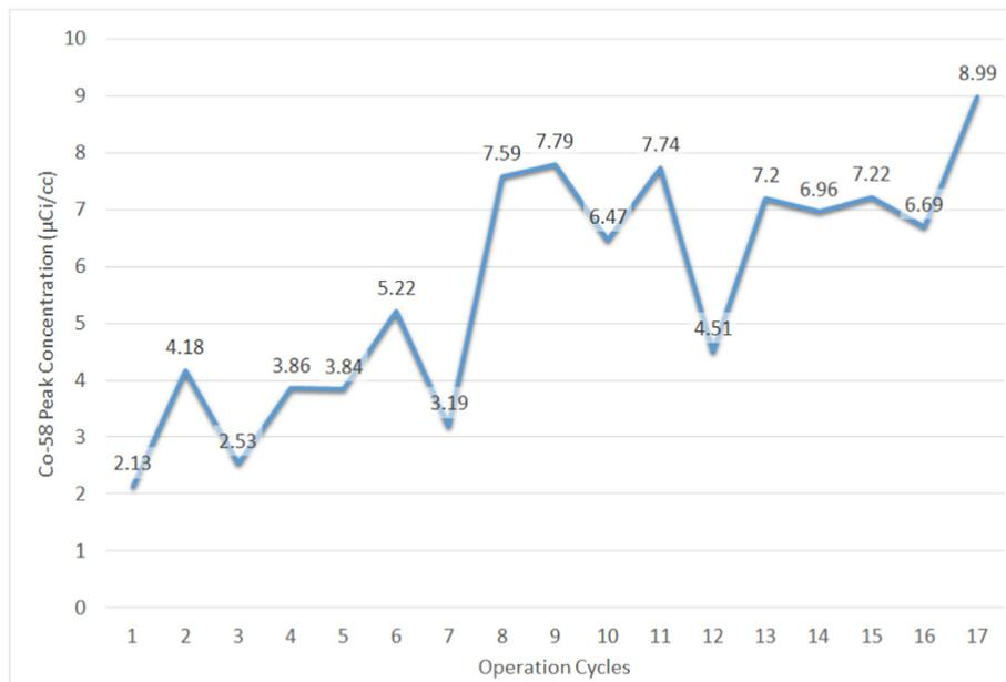
Fig. 3. Co-58 peak data during shutdown chemistry at the NPP.
