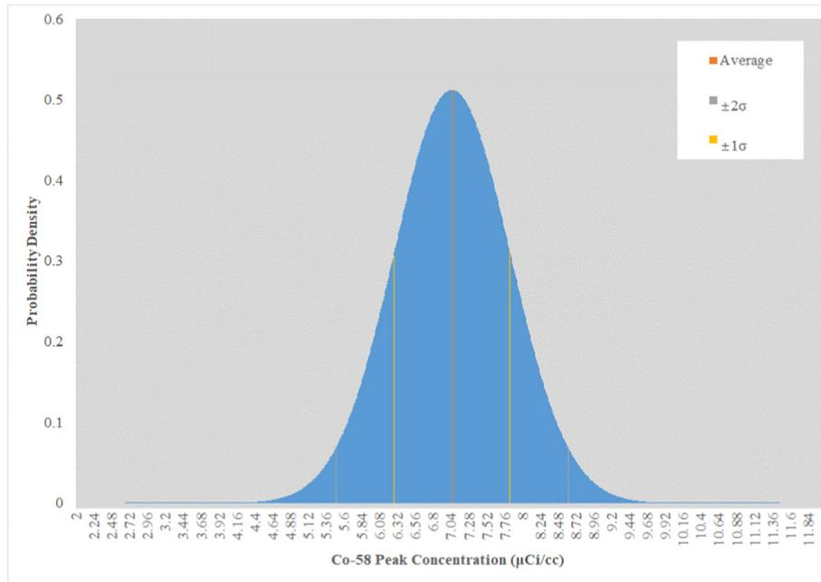
**Fig. 4.** Standard normal distribution for Co-58 peak data during shutdown chemistry at the NPP.
