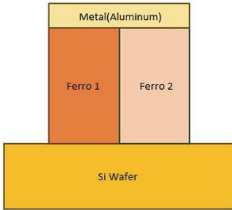
Fig. 1. Double Ferroelectric-RAM structure for Multi-level states.
