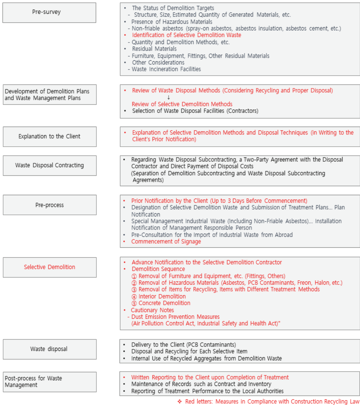
Fig. 2. Demolition process for selective demolition in accordance with the Japanese construction recycling law
