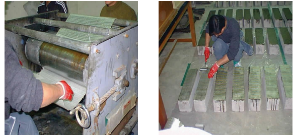
(a) Composite saturation (b) Priming and restrengthening
