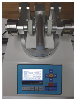
Fig. 6 Taber abrasion test on antifouling coating agent
