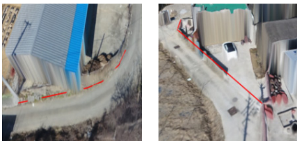
<Figure 8> Fence Line Finalization using 3D Image
