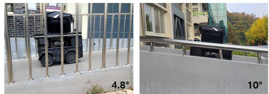
Fig. 6 Ramp climbing test
