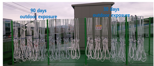
[Figure 2] Fiber rope outdoor exposure
