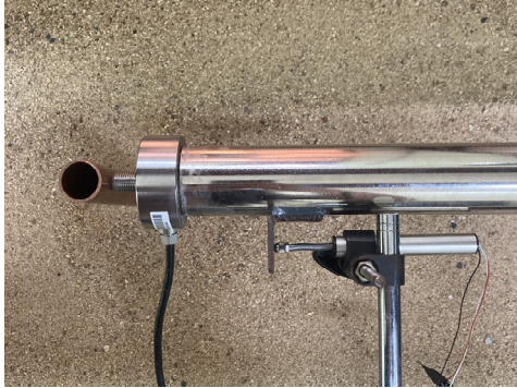
(c) Setting displacement meter, load gauge
