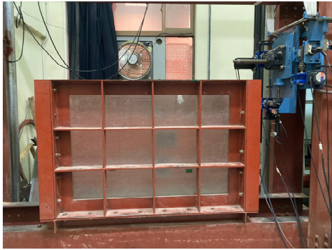
(a) Forming the model ground, put in the model pile vertically
