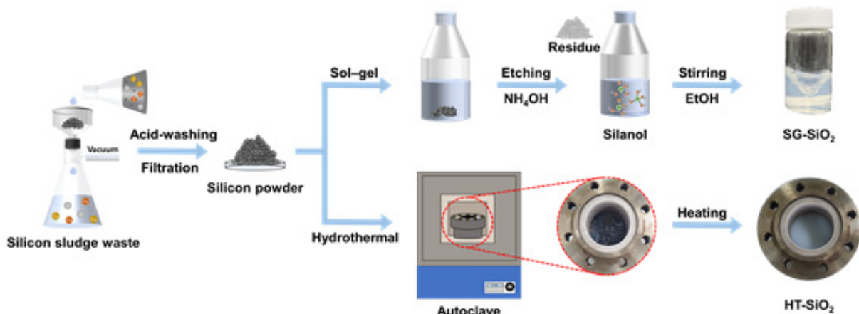
Fig. 1. Schematic illustration for synthesis of silica nanoparticles using sol-gel and hydrothermal method employing silicon sludge waste.
