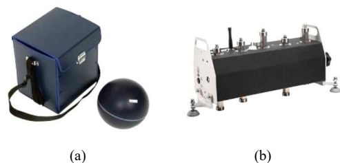
Fig. 6. Heavy & light weight impact sources. (a) Rubber ball, (b) tapping machine.
