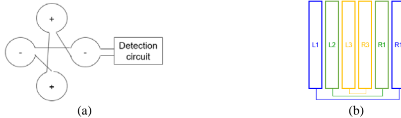
Fig. 2. Layout of passive detection-only coil sets. (a) a balanced coil set [22] and (b) symmetric coil sets [20]
