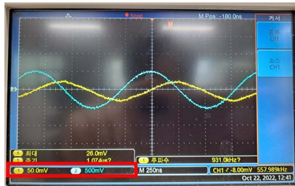
Fig. 11. Voltage signals when there is no MO. Channel 1(yellow line, 50 mV/div): voltage measured at the node between the resistor and the capacitor, and channel 2(blue line, 500 mV/div): voltage measured at the node between the capacitor and the coil.
