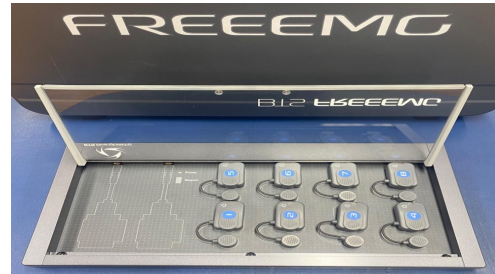
Figure 3. Surface EMG (BTS Free EMG)
