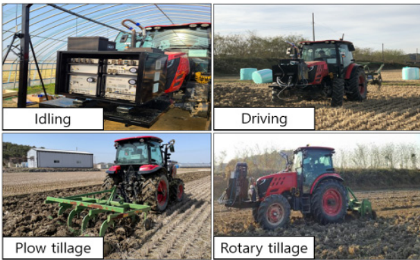
Fig. 4 Field experiment of the tractor for measuring exhaust gas emissions
