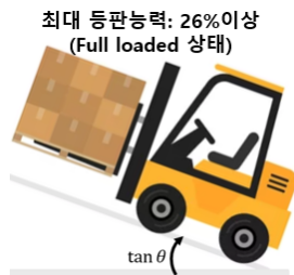
Fig. 1 Forklift max. grade ability
