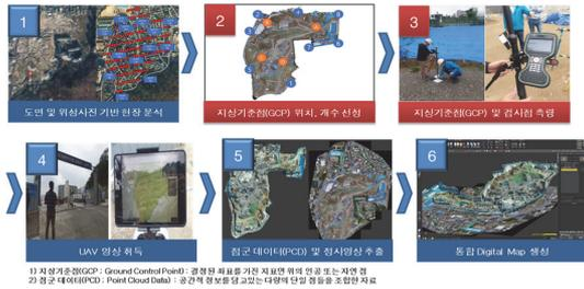
Fig. 1 Digital map generation of construction site using drones
