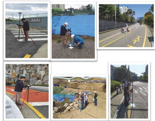
Fig. 2 Ground Control Points(GCPs) survey
