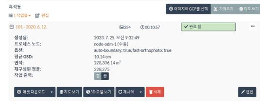
(b) orthographic image process (WebODM 1.9.19 fast-orthophoto)
