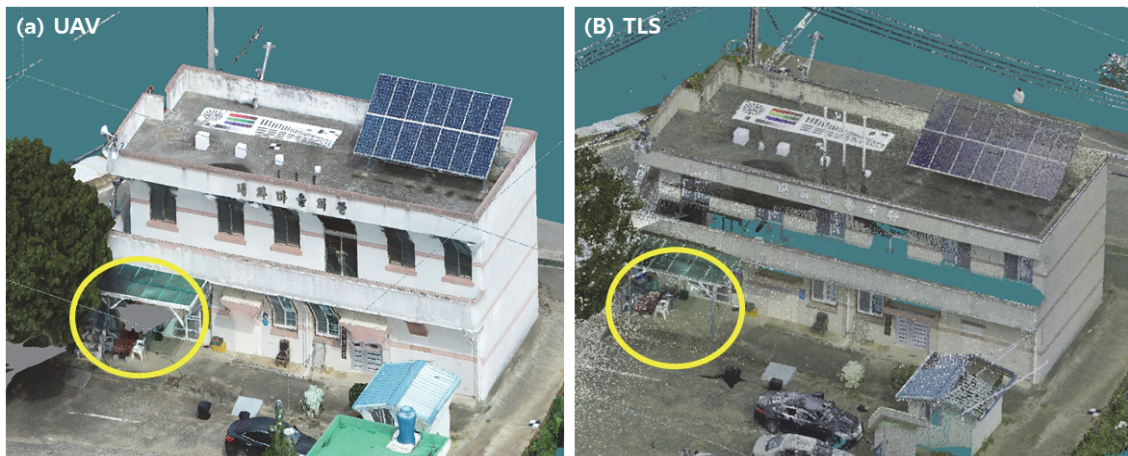
Fig. 8 Pointcloud generation error part by data acquisition method
