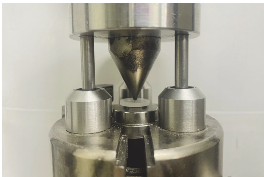
Fig. 3 Configuration of piston-on-3-ball biaxial flexural strength test
