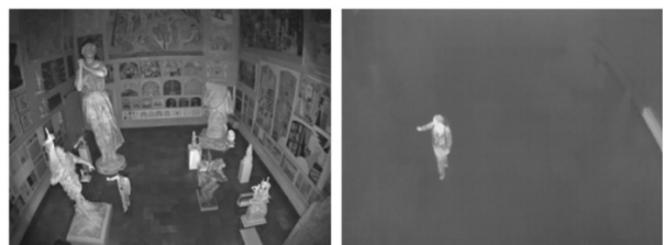
[Fig. 2] Laser IR Image and Thermal Sensing IR Image [9]
