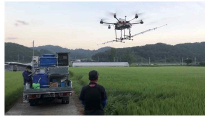
Fig. 4. Drone for spraying agricultural chemicals
