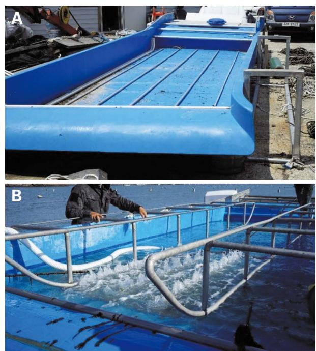
**Fig. 1.** Installation of air bubble device in activating treatment tank. A. Set up an air bubble line in the tank, B. Image of drive on air bubble device.
