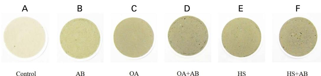
**Fig. 4.** Images of foreign matter after membrane filtration treated seawater with different activating treatment agents and an air bubble device treated. A. control, B. air bubble device (AB), C. organic acid activating treatment agent (OA), D. organic acid activating treatment agent with an air bubble device (OA + AB), E. highly saline solution (HS), F. highly saline solution with an air bubble device (HS + AB).
