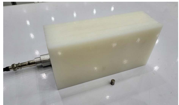
Fig. 5. 3 He chamber, moderator and 252 Cf calibration source.
