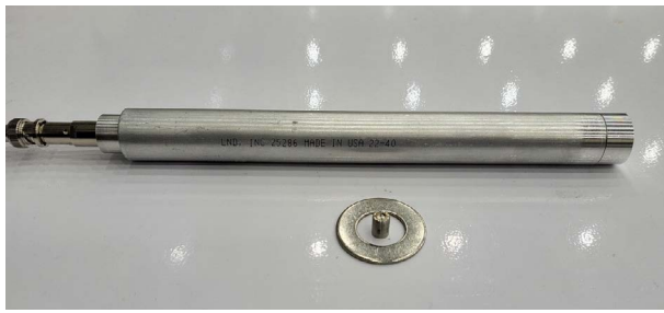
Fig. 3. 3 He chamber and 252 Cf calibration source.
