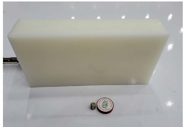
Fig. 8. ^3\text{He} chamber, moderator, ^{252}\text{Cf} and ^{137}\text{Cs} calibration sources.
