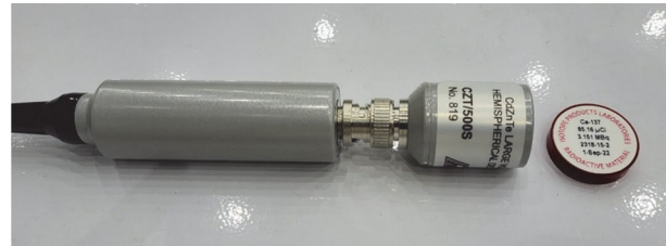
Fig. 3. CZT sensor and ^{137}\text{Cs} calibration source.
