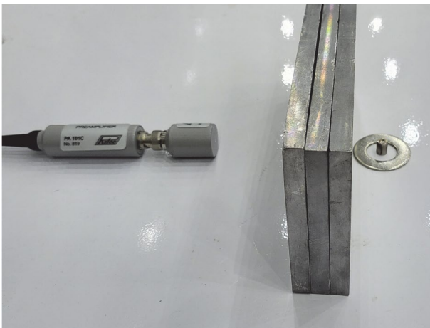
Fig. 7. CZT sensor, Lead Shield and 137 Cs calibration source.
