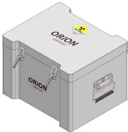
Fig. 5. Transport container full model for structure analysis.
