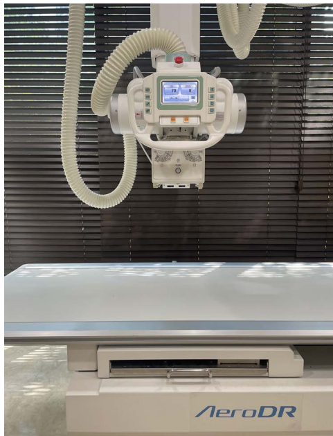
Fig. 3. X-ray generator model (DigiRAD-FPC R-1000-150, SITEC, Korea).
