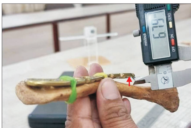
Fig. 4. Showing vertical gap between the bone and plate at the medial end of the clavicle. The gap is indicated by red arrow.
