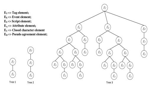
Fig. 2. Attack vector basic element succession Figure
