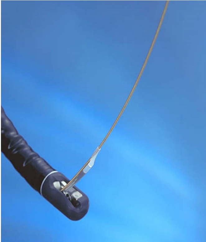
Fig. 1. A thin caliber intraductal ultrasonic probe. The diameter of the transducer (UM-G20-29R; Olympus Co., Ltd.) is 2.4 mm, the frequency is 20 MHz, the axial resolution is 0.1 mm, and the maximum transmission distance is about 20 mm.
