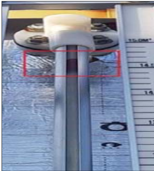
Fig. 2. Level gauge and Level indicator.
