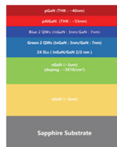
Fig. 2. Epitaxial layer structure.
