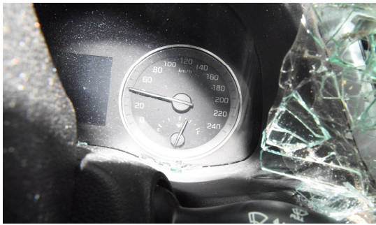
Fig. 7 Speed indication within the instrument cluster
