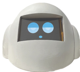
[Fig. 1] The prototype robot with 4 inch display (robot size: 21 cm × 18 cm × 12 cm)
