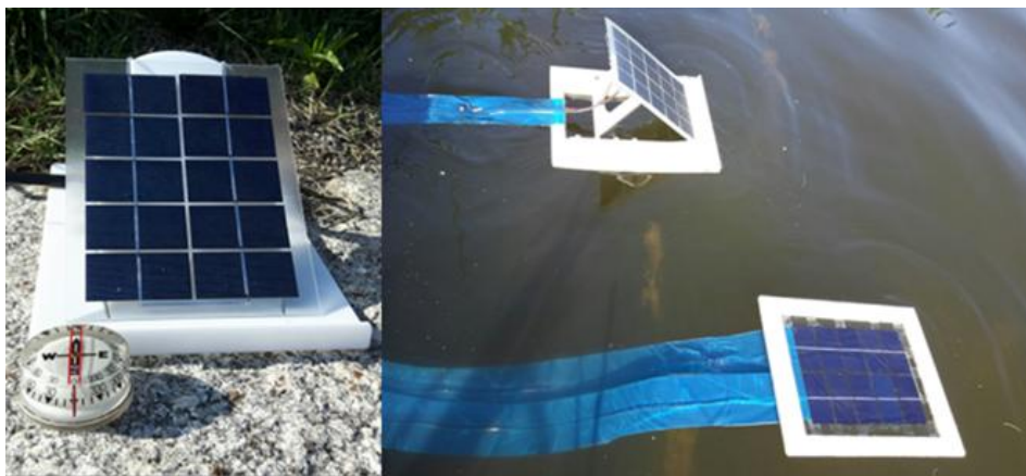
Figure 1. Three cells under experiments (left : ground cell, top : water platform cell, bottom : floating horizontal cell)
