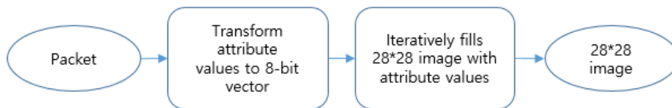
Figure 2. Image generation based on Direct conversion
