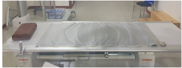
Fig. 4. The figure above is the heating mat made of carbon fiber.
