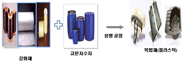
Fig. 2. The figure above shows the process of making carbon composites using reinforcing materials and polymer materials.
