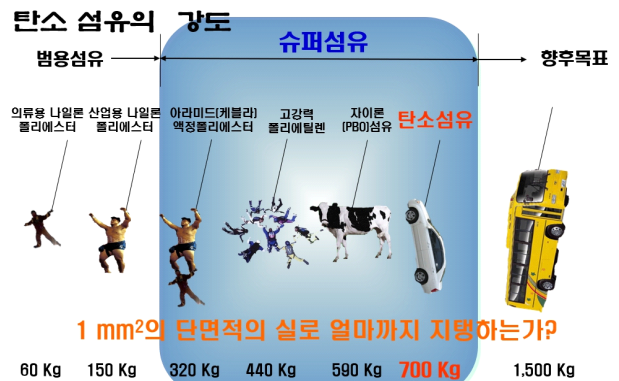
Fig. 1. How many kilograms do you weigh with a 1 mm 2 thread. It can support 700 kg with 1 mm 2 carbon fiber.
