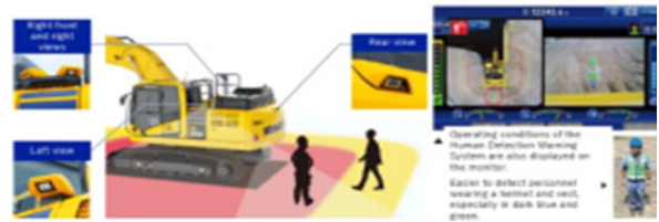
Fig. 7 Sensing angle of automobiles and construction machinery
