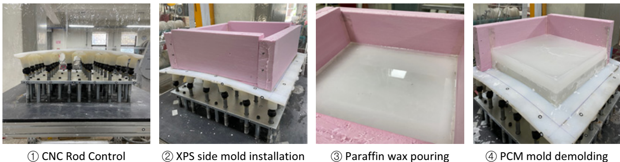
Figure 4. PCM mold manufacturing process
