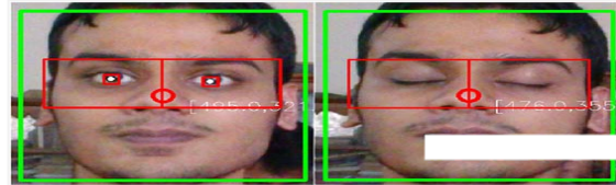
Figure 13 Camera based Eye-blink detection.
