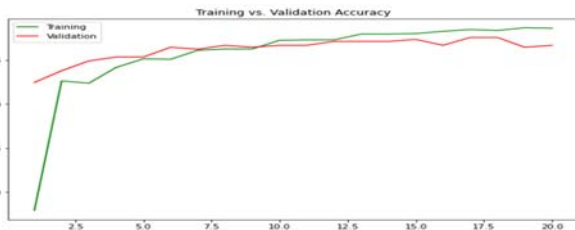
Fig 47 DenseNet201 training vs validation accuracy with SGD optimizer
