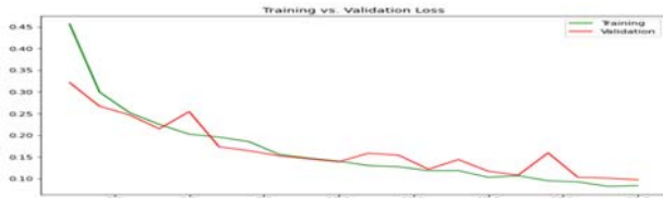
Fig 28 InceptionResNetV2 training vs validation loss with SGD optimizer
