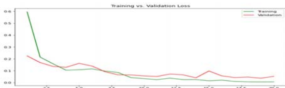
Fig 22 InceptionResNetV2 training vs validation loss with Adam optimizer
