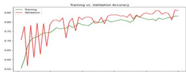
Fig 20 VGG19 training vs validation accuracy with SGD optimizer
