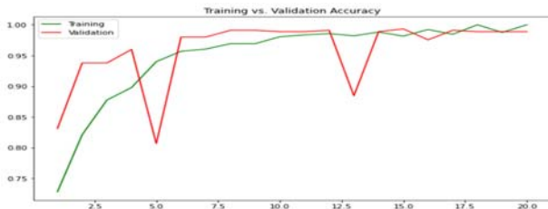
Fig 35 Inception training vs validation accuracy with RMSprop optimizer
