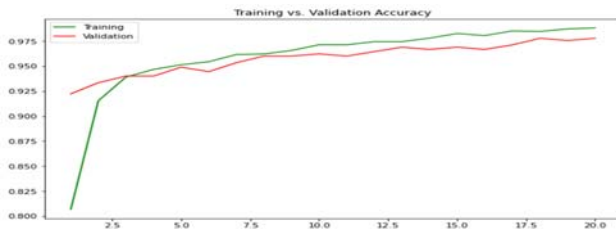
Fig 11 MobileNet training vs validation accuracy with SGD optimizer
