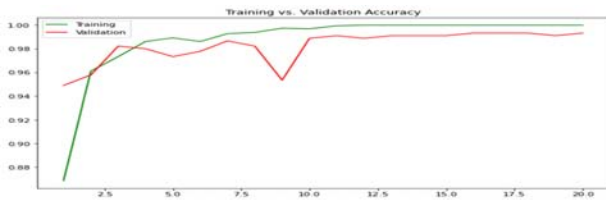
Fig 41 DenseNet201 training vs validation accuracy with Adam optimizer
