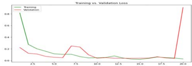
Fig 43 DenseNet201 training vs validation loss with Rmsprop optimizer
