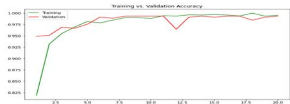
Fig 8 MobileNet training vs validation accuracy with RMSprop optimizer
