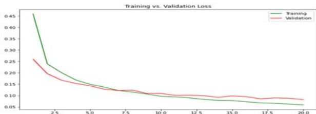
Fig 46 DenseNet201 training vs validation loss with SGD optimizer
