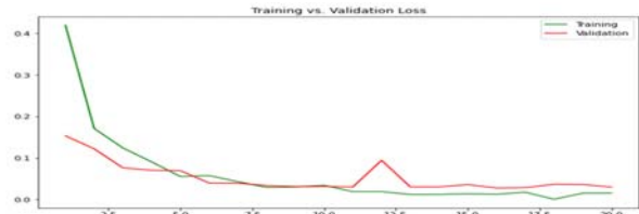
Fig 7 MobileNet training vs validation loss with RMSprop optimizer
