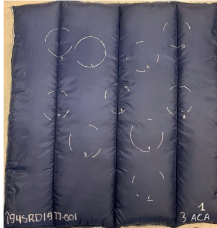
Location of the ten measurement spots to determine the average air permeability of assemblies
