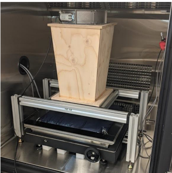
Fig. 2. Wind tunnel designed to generate a vertical airflow at a controlled speed simulating wind.
