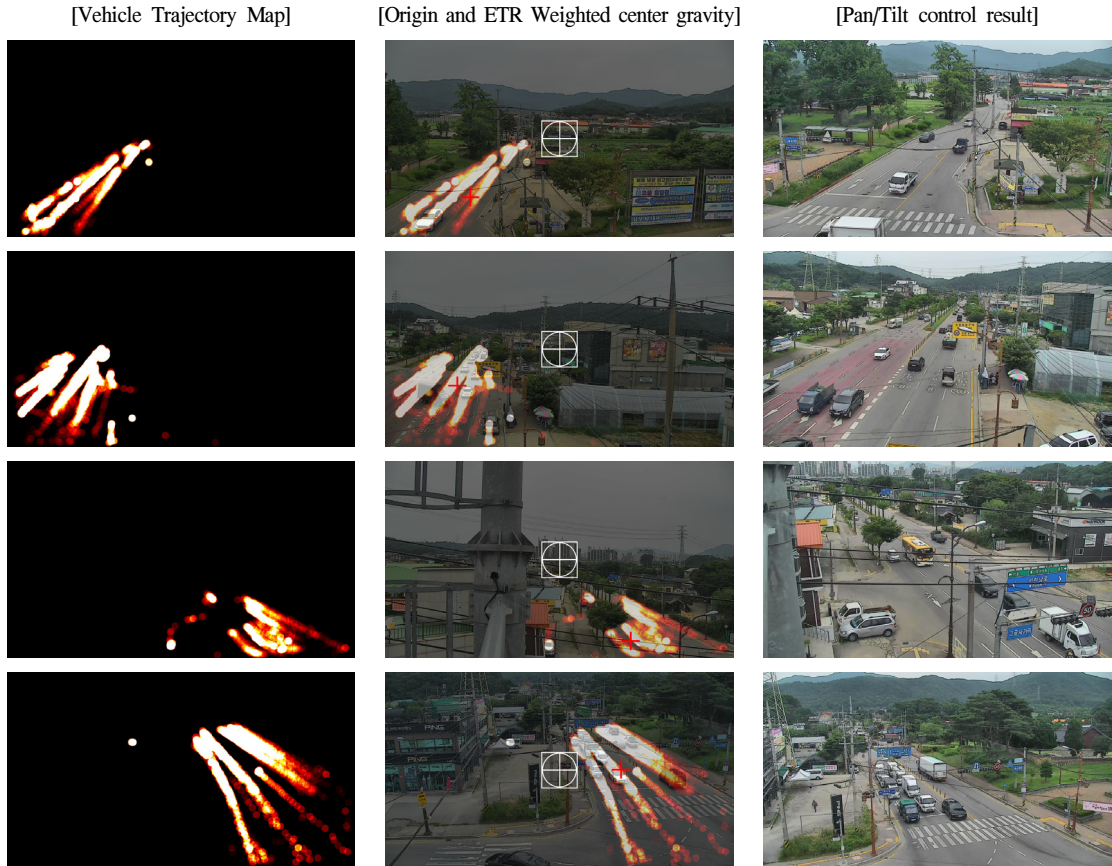
<Fig. 6> PTZ control result through vehicle trajectory analysis
