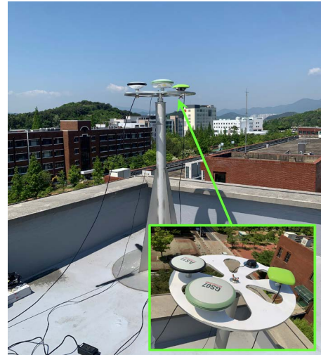
Fig. 2. Set up of temporary station with different grades of receiver to obtain data set B.
