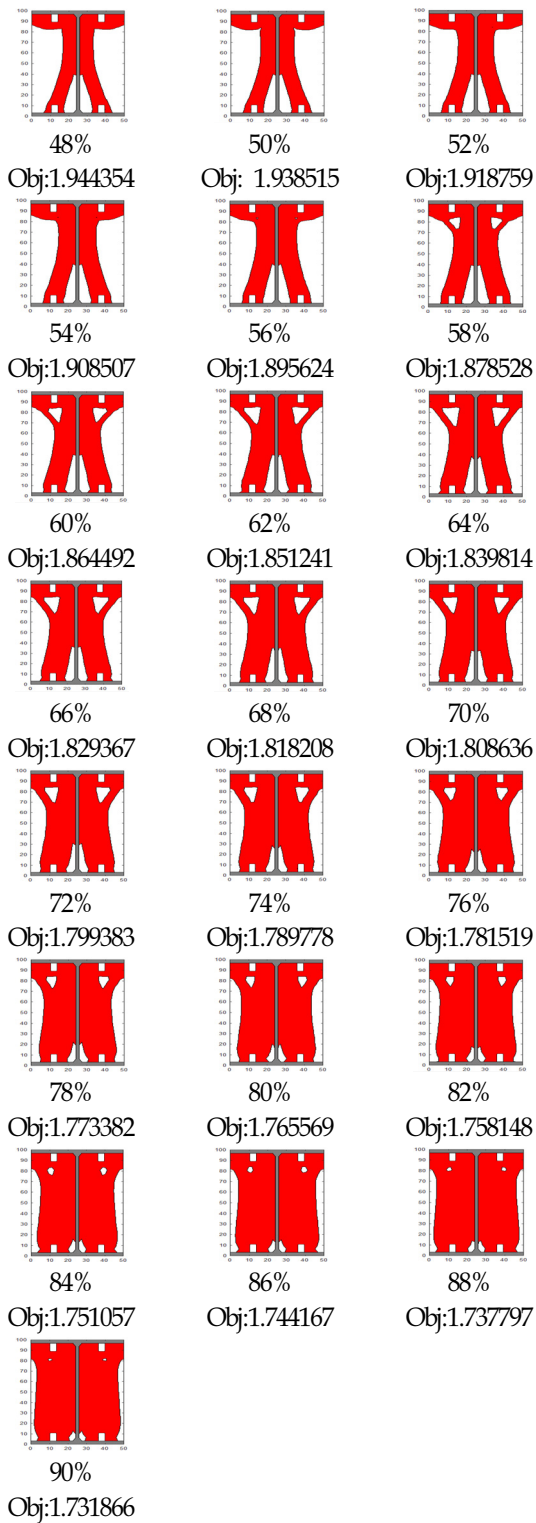
<Fig. 6> #2, 100×50×2×3 optimal topology configuration in terms of volume fraction
